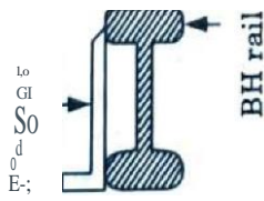
Straight cut switch Fig. 2.M.2.
